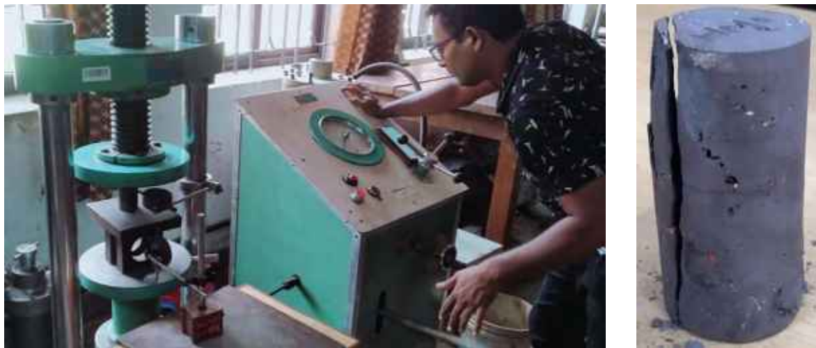
Figure V. Determining UCS of rock sample
