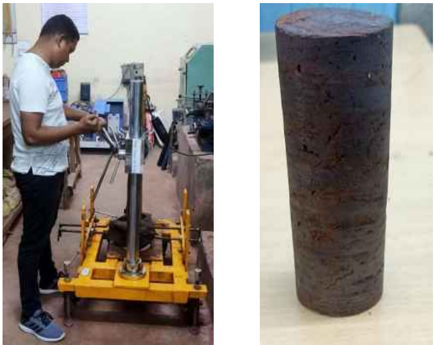
Figure IV. Coring operation and cored specimen
